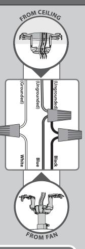
Turn the splices upward and push them carefully back through the hanger bracket into the outlet box. Spread the wires apart, with the grounded wires on one side of the outlet box and the ungrounded wires on the other side of the outlet box.
